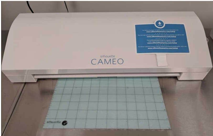
Figure 1: Silhouette Cameo® cutting machine and “sticky mat” for holding PDMS sheets in place.
