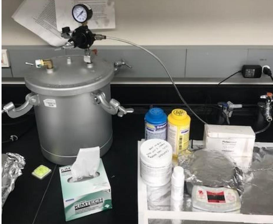
**Required setup for Smoothcast molds**
