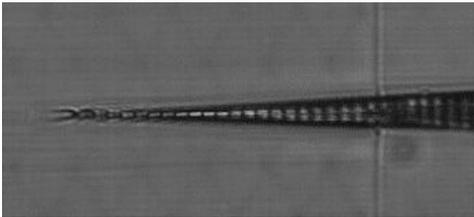
Serrations: 5  $\mu\text{m}$  wide, 2  $\mu\text{m}$  deep. Serrations don't come out at 25x (resolution is 3  $\mu\text{m}$  )
