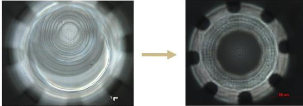
Figure 6. An off-center issue could be avoided by combine two GWL files with a different writing direction.
