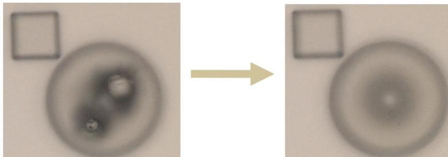
Figure 2. Preheat is a useful tip to reduce bubble formation in writing.
