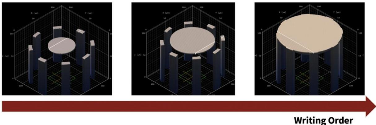
Figure 4. An illustration of explaining why normal writing order cause off-center issue for the overhanging structures.
