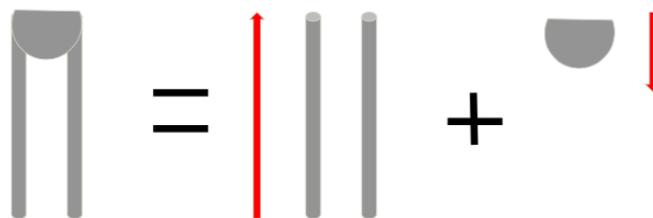
Figure 5. An illustration of writing direction strategy for an overhanging structure.
