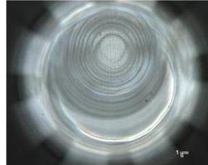
Figure 3. Off-center printing issue for a overhanging structures.
