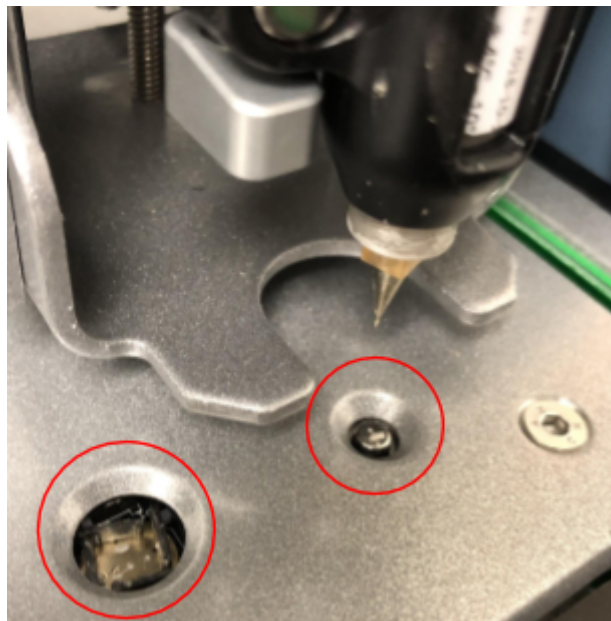
Figure 7: Limit switches (circled in red) should be cleaned with a Q-tip after every print to prevent inaccurate homing and positioning.
