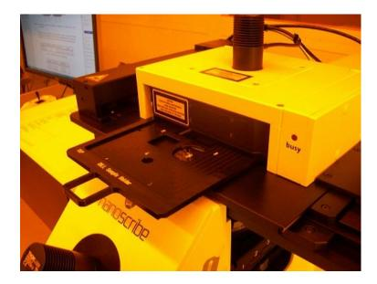
4. Make sure that the sample holder is set at the right position (when the sample holder is inserted, you can hear a "click")
