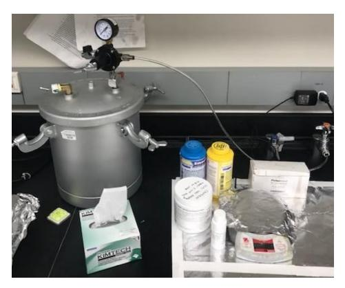
**Required setup for Smoothcast molds**
