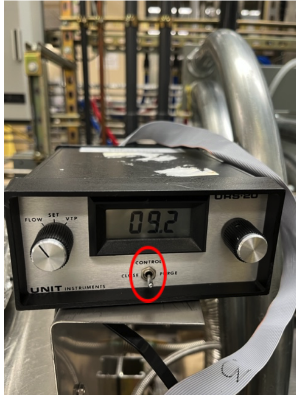
Figure 1: MFC Controller Must be in “Control” Position During ZnO Deposition
