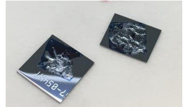
PMMA/graphene on GaAs (SC2 was very violent)
