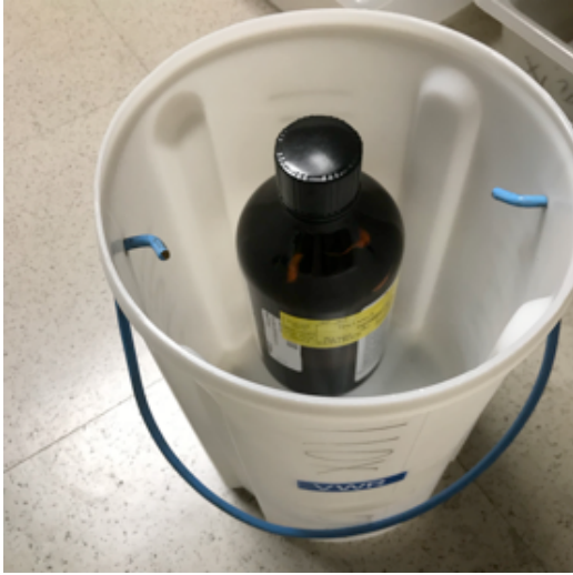
Figure 2. Chemicals in a secondary container bucket.
