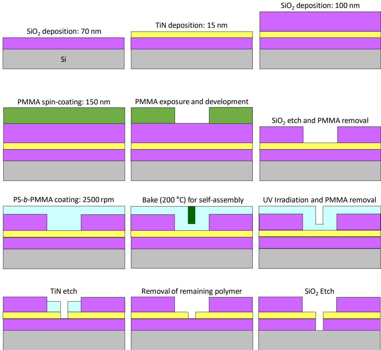
Figure 2: Diagram of full process for SiO 2 /TiN guiding well fabrication, directed self-assembly, and pattern transfer into TiN and SiO 2 .
