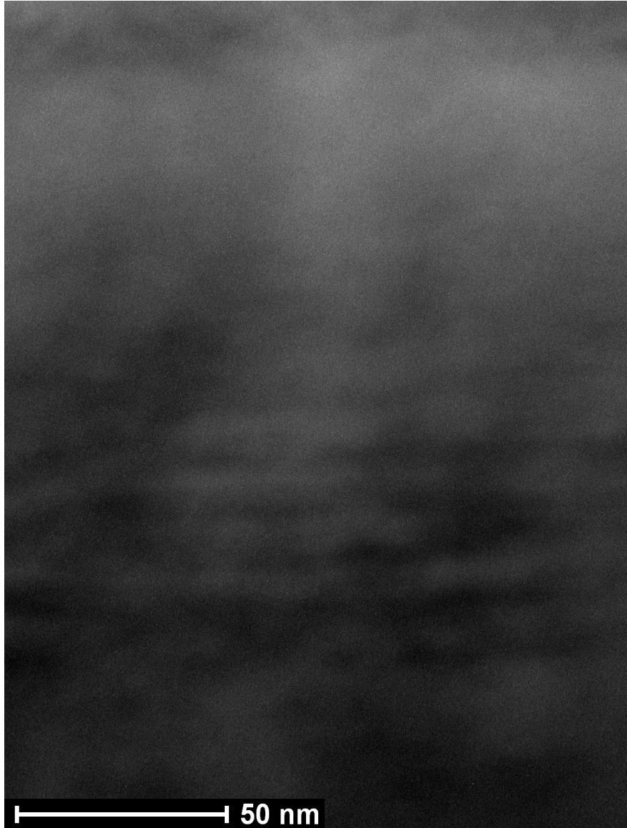
Figure 4: The MQWs show gross well width fluctuations, though a more careful TEM study would be necessary to improve confidence.
