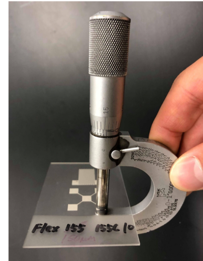
Thickness measurement with micrometer
