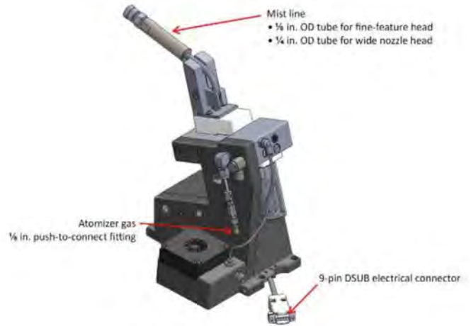
Figure 52. UA Max atomizer connections
