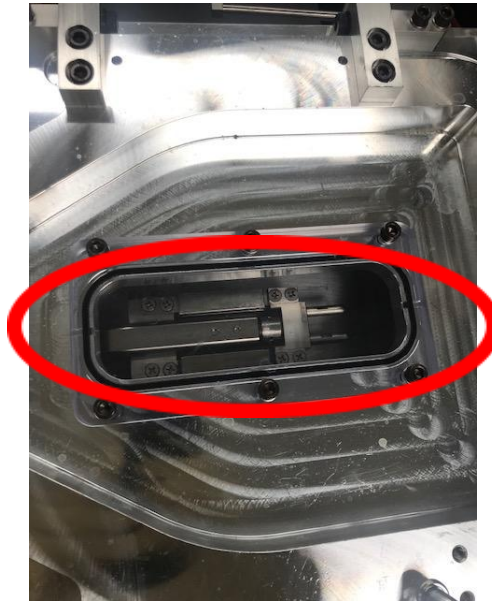
Figure 2: View of transfer fork through loadlock window
