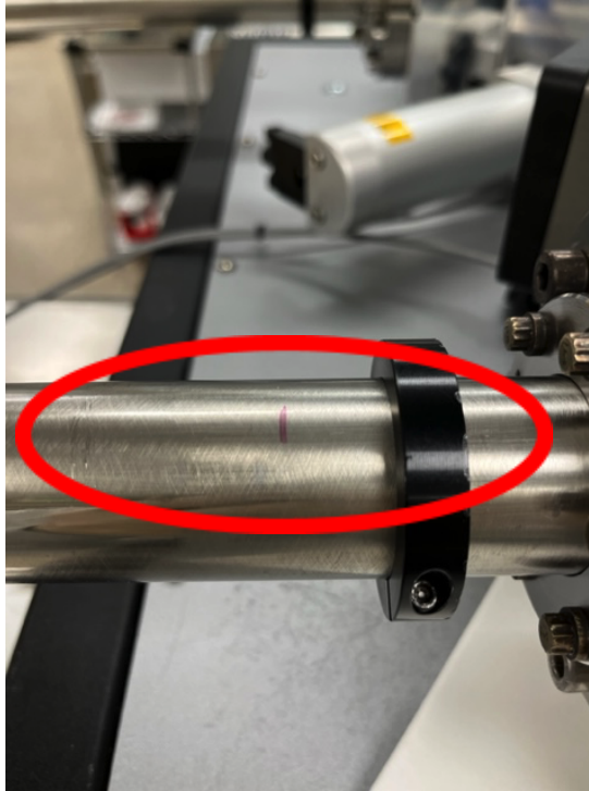
Figure 3: Mark indicating full fork engagement. The front of the black sleeve must reach this line. The mark is drawn in Sharpie, and may change colors
