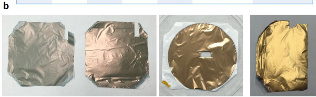
Figure 3. (a) Parameter for Au sputtered on PE and (b) optical images of different size.
