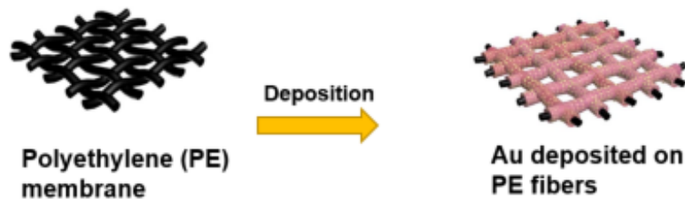
Figure 2. Scheme of gold sputtered to polyethylene
