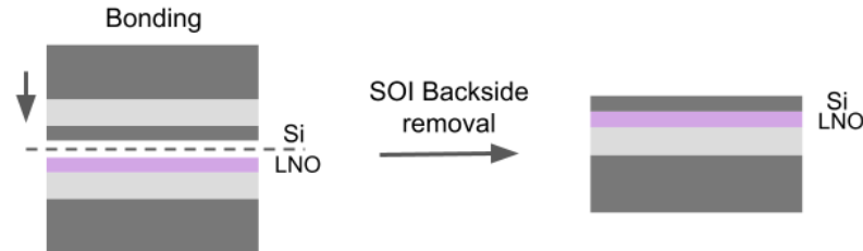
Figure 1. Schematic depicting the bonding and backside removal steps, resulting in a Si thin film sitting on a LNO thin film.
