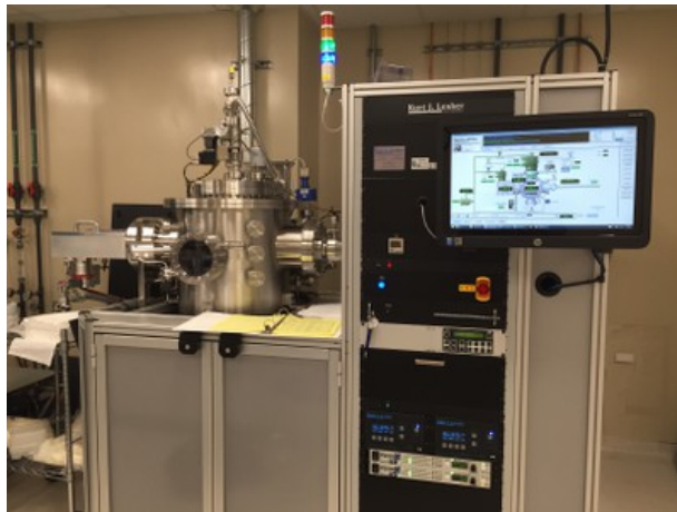
Figure 1. Lesker Sputter, the sputtering instrument in the Exfab facilities
