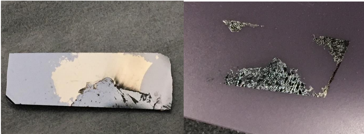
Figure 38: Substrate (left) and epilayer on thermal release tape (right) after exfoliation.
