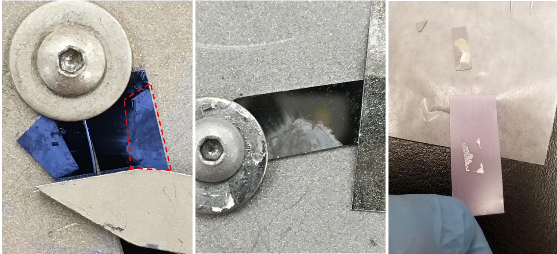
Figure 37. Left: Sample G6y mounted on the AJA chuck before evaporation (sample on the right), showing the as-grown surface after MOCVD. The rougher region (outlined in red) is the graphene area. Center: After deposition of the Ti/Ni stressor layer (a problem with the evaporator required the samples to be unloaded and mounted again). Right: Substrate and the exfoliated epilayer immediately after the tape is peeled off. Area on the left part of the tape corresponds to the graphene region.
