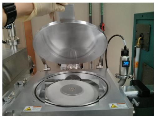
2) Hold chuck from the backside and remove from load lock.
